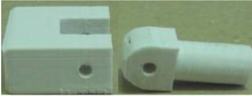
Figure 9 - A Watford Grammar School sixth form group investigated calculus relating to velocity, height and distance of a projectile. A device that had previously been used had become unreliable and a coupling was produced on the 3D printer to hold the internal catapult. A series of projectiles were then produced for the project using the 3D Printer.
