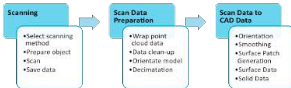
Figure 1: Workflow for scanning an object
